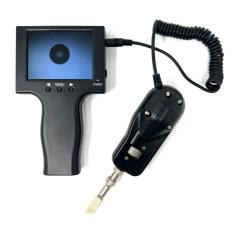
QT-FOVIM-HH-LCD-4X Fiber Video Microscope can offer 600 magnification for the fibers of 125um(diameter), single-mode and multi-mode are all included. (based on **the magnification of the 9 inch display, which can inspect** 685000um end-face.) The enlarged picture is then sent to the display through a video signal. Consequently the status of fiber end-face is showed clearly.
